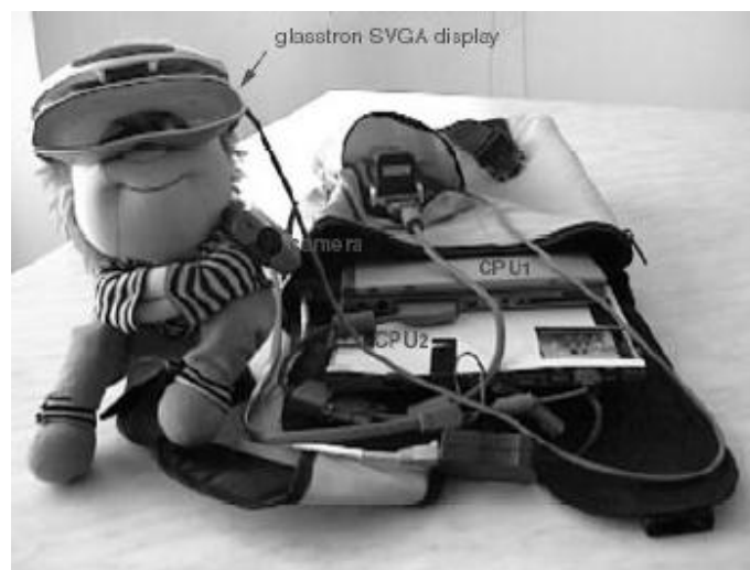
Figure 15 Wearable Cinema setup:backpack, two CPUs, camera and lightweight color SVGA glasstron display (Sparacino, Davenport et al. 2000)
